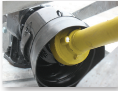
Splined input shaft Slip clutch Standard.
