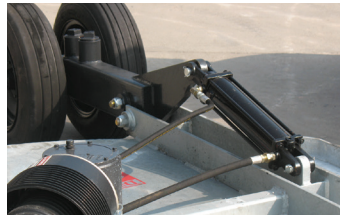
Our updated hydraulic phasing level lift system is a superior improvement over the outdated mechanical lift system.
